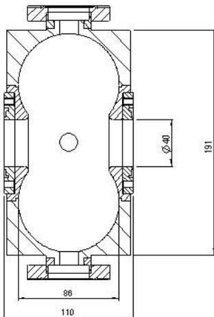
Figure 3: The RF cavity model
