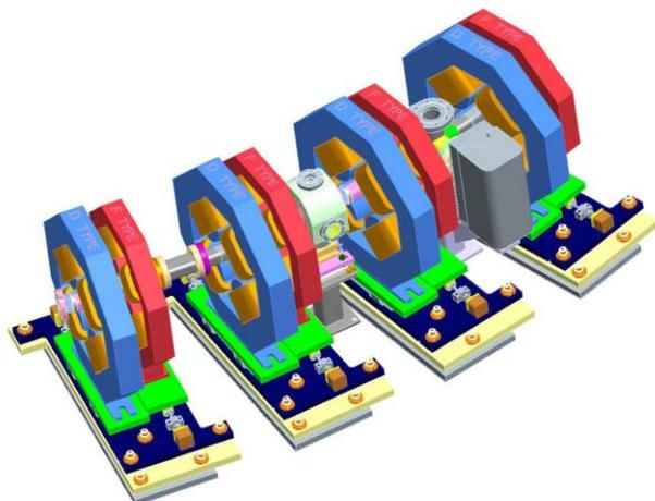
Figure 1: Four EMMA cells, showing the magnets mounted on sliders. Between the middle two cells is an RF cavity. The left gap has a resistive wall monitor and the right an ion pump.
