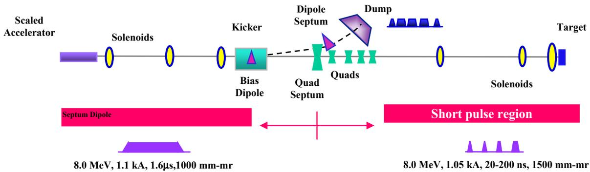
Figure 1: Schematic layout of DARHT 2<sup>nd</sup> Axis scaled accelerator downstream transport.
