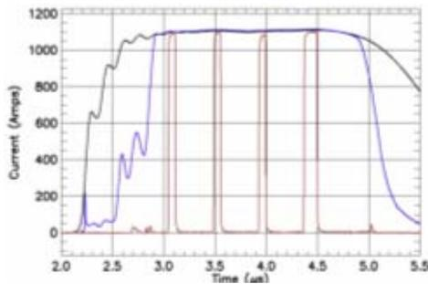
Figure 4: Beam current profile at injector, accelerator exit and target showing four kicked pulses.
