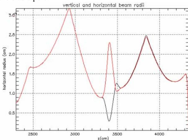
Figure 2: Beam envelope in the downstream transport.
