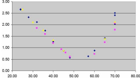
Figure 5: Beam size vs. magnet current for kicked beam.
