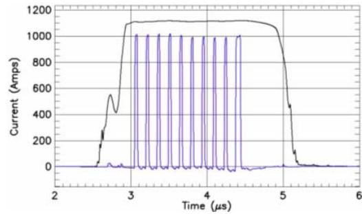
Figure 6: Kicker pulse format for beam desorption study.
