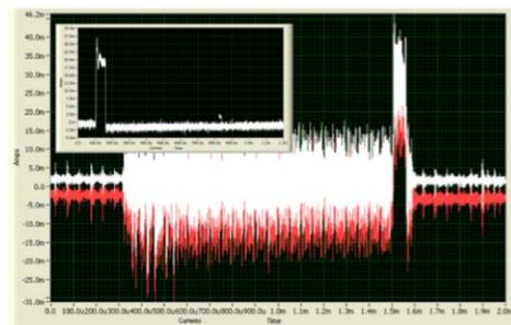
Figure 4: The worst-case signal: DTL BCM200. The insert shows a much cleaner signal from CCL BCM102.
