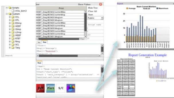
Figure 3: A web-based interface in JavaScript to acquire, process, and publish accelerator data. To the right is the web graph (top) and report (bottom). This version uses the MySQL database and PHP for server side functions.
