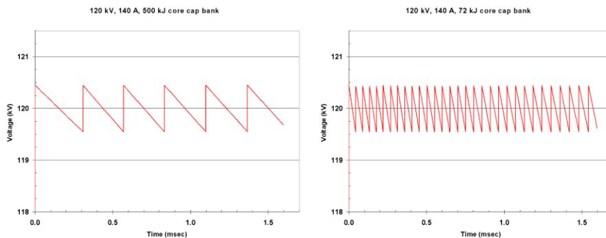
Figure 3. (left) A very large capacitor bank has a low droop rate, and needs few correction pulses. (right) A smaller capacitor bank droops quickly, so many more correction steps are required.
