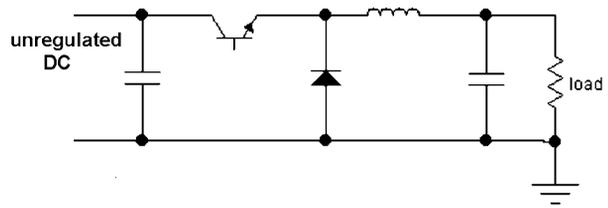
Figure 4. The basic architecture of a switching buck regulator, or DC-DC down-converter, shows the series switch, the freewheeling diode, and the filter inductor.
