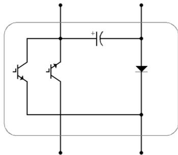
Figure 2. Unit Marx cell, showing pulse switch (at left) and recharge switch (center).
