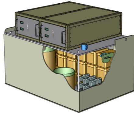
Figure 1. Proposed ILC Marx modulator, nominally delivering 125 kV, 140 A, 1.5 ms, 5 Hz – from a raw 3-phase 13.8 kV input.
