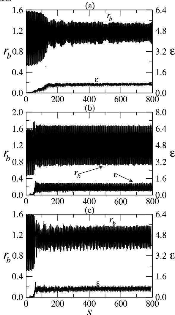
Figure 2: Emittance  $\varepsilon(s)$  growth and envelope  $r_b(s)$  dynamics in: (a) full simulations, (b) the case where the core  $r_c(s)$  oscillates with fixed amplitude, and (c) in the self-consistent simplified model.
