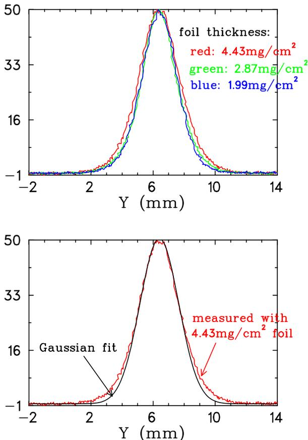
Figure 2: Top: The measured vertical profile of beam on monitor VM6 for 3 stripper foils of different thicknesses. The difference between 4.43 and 2.87 mg/cm<sup>2</sup> foils being relatively larger is because the multiple scattering in the 4.43 mg/cm<sup>2</sup> foil dominates the emittance. Bottom: A comparison between the measured profile and a Gaussian distribution. The core is just a Gaussian and the tails are due to the large angle scattering.
