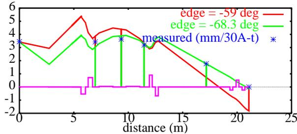
Figure 4: Beam centroid shift (in mm) measured vertically up to the monitor VM6 and the trajectory fitted. The vertical lines represent the location of the monitors. The fit with edge angle  $-59^\circ$  is not good, but the fitted  $-68.3^\circ$  angle is satisfactory.
