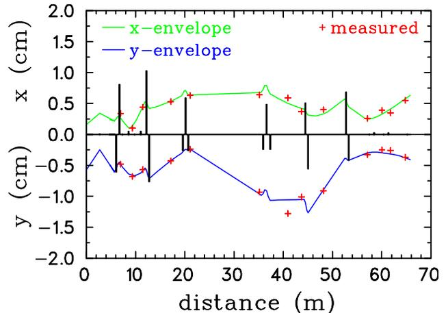
Figure 5: Measured and calculated beam sizes agree very well in the whole beamline. A total of 6 parameters were fitted to obtain the best fit.
