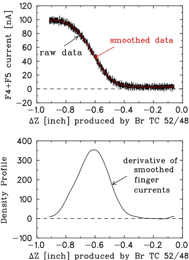
Figure 3: Top: HE1 probe measured finger currents sum (F4+F5) vs. the vertical position of the beam. Bottom: vertical distribution of the beam, derived by differentiating the current sum (F4+F5) w.r.t. the vertical position Z.
