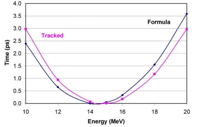
Figure 3: Energy variation of time of flight in one cell.
