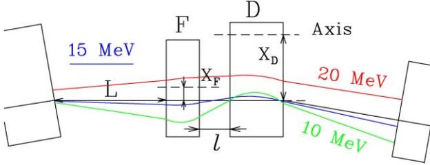
Figure 2: Orbits in a quadrupole doublet cell.
