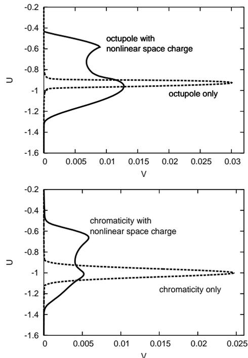
Figure 1: Stability diagrams obtained with the dispersion relation Eq. (2). Top: for an octupole only and for a combination of this octupole with nonlinear space charge (waterbag distribution); bottom: for the chromaticity effect only and for the combination with nonlinear space charge.
