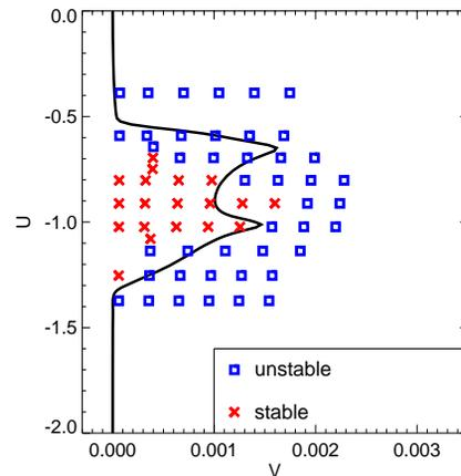
Figure 3: Combination of chromatic effects and nonlinear space charge.
