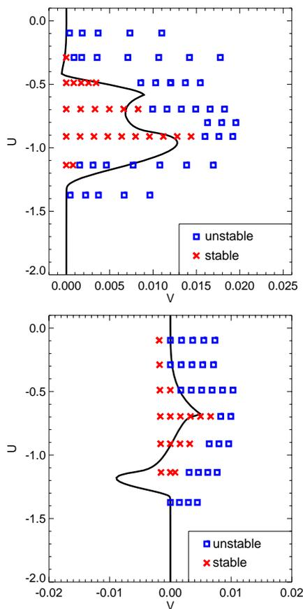
Figure 2: Combination of nonlinear space-charge and an octupole with the advantageous polarity (top), disadvantageous polarity (bottom). The symbols are the results of simulations, the lines are stability boundaries from the dispersion relation.
