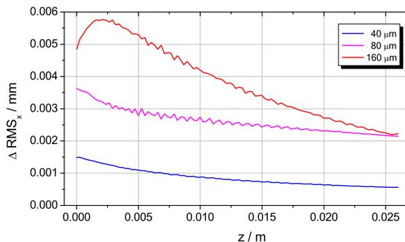
Figure 3: Differences in the transverse RMS bunch size for different transverse mesh step sizes with respect to the results obtained for a transverse step size of 20  $\mu\text{m}$ .
