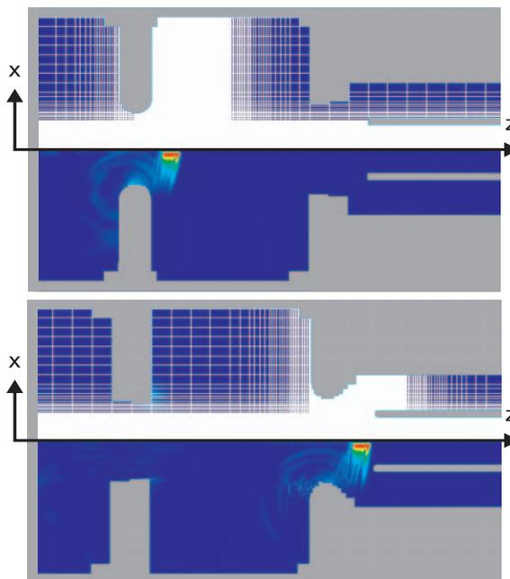
Figure 1: Combined view of the computational grid and the computed space charge fields at two instants in time for a simulation of the PITZ [8] gun (x-z cut).
