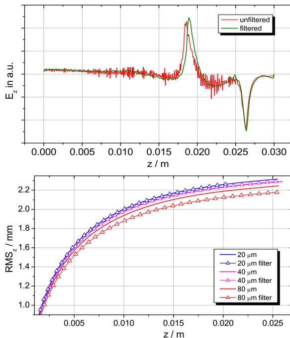
Figure 5: Effect of spatial current filtering on the excited electric field (top) and on the bunch length (bottom).
