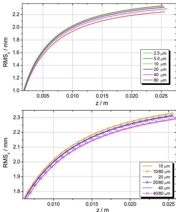
Figure 2: Convergence of the RMS bunch length with respect to the longitudinal mesh step size for an equidistant mesh (top). RMS bunch length for static mesh refinements up to a distance of 1 cm from the cathode by factors of 2 to 16 (bottom).
