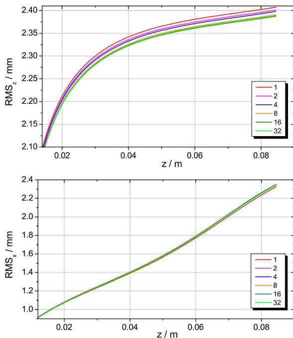
Figure 4: Computed longitudinal and transverse bunch size depending on the number of emission samples per cell.
