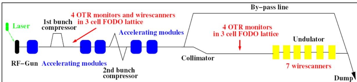
Figure 1. Schematic layout of FLASH (not to scale). Total length is about 250 m. Locations of the diagnostic sections for emittance measurements are indicated.
