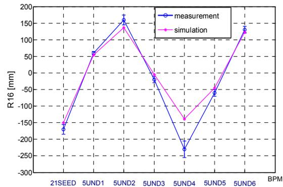
Figure 3: Measured and simulated  $R_{16}$  in the undulator.
