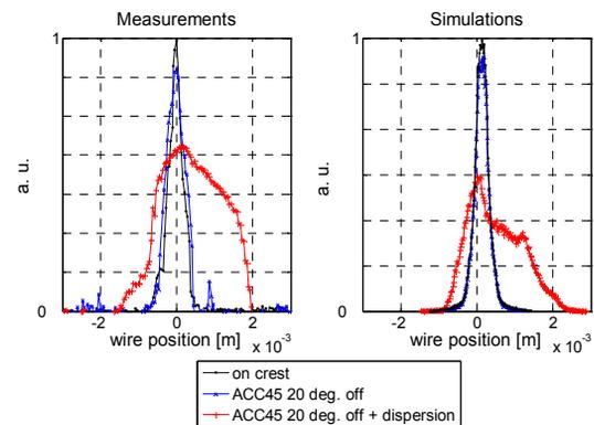
Figure 4: Measured (left) and simulated (right) beam profiles at the wire-scanner 5UND6.
