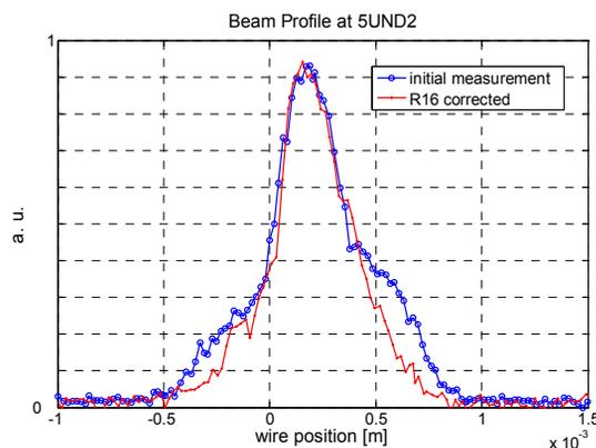
Figure 6: Beam profile measurement at wire-scanner 5UND2 before and after dispersion correction.
