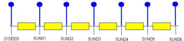
Figure 2: Undulator section sketch. The wire-scanner stations are indicated.
