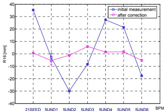
Figure 5:  $R_{16}$  in the undulator before and after dispersion correction.
