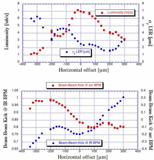
Figure 3: Horizontal offset scan done on June 9h 2004 with a finite crossing angle of  $\pm 11\text{mrad}$ . Beam currents were 940mA and 1200mA for HER and LER, respectively. The number of bunches was 1289 for each ring and the averaged bunch spacing was 3.77 RF buckets. The luminosity, the LER vertical beam size and the horizontal beam-beam kick were recorded. Two different methods of the horizontal offset measurements were utilized.
