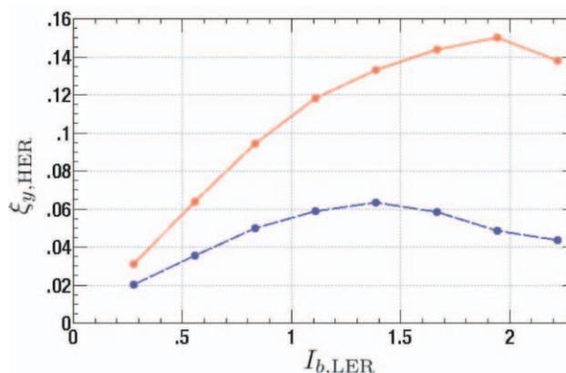
Figure 1: Enhancement of the vertical beam-beam parameter by a head-on (crab) collision (upper curve) comparing with the crossing angle of  $\pm 11\text{mrad}$  (lower curve), obtained by a strong-strong beam-beam simulation. Parameters are the same as the present KEKB.
