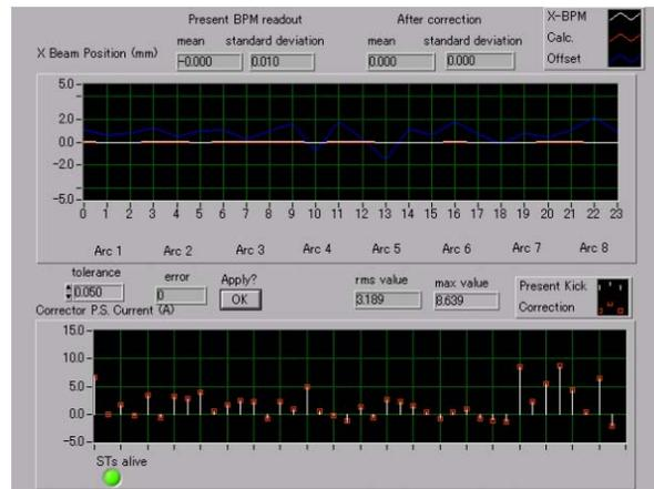
Figure 4: A snap shot of the COD correction GUI running on the control PC. Upper graph shows the BPM readout (white line), expected orbit after COD correction (red line) and BPM offset (blue line). Bottom graph shows the present strengths of the steering magnets (white bars) and calculated strengths for the next correction (red squares).
