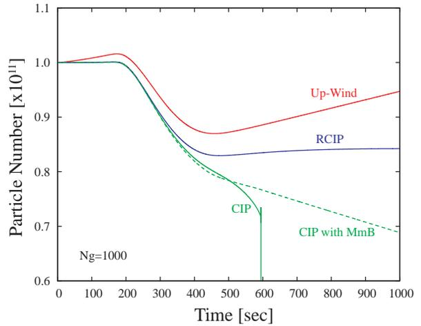
Figure 5: Particle number at each calculation method for the conservation law check.
