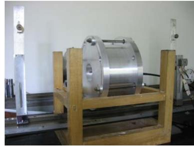
Figure 2: Picture of the 2-half-cell assembly and bead-pull system
