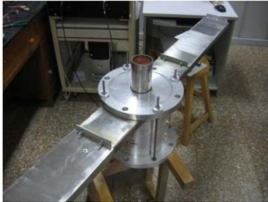
Figure 4: Picture of the cold model with damping waveguide
