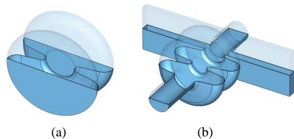
Figure 1: Simulated design (a): 2-half-cell (b): 2 cell cavity with damping waveguide
