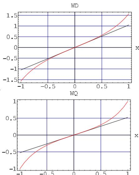
Figure 1: Dipole (left) and quadrupole (right) components of the wake field as a function of  $x_0/g$ ,  $x = 0$  and  $x_0 = 0$ ,  $x/g$  respectively, for  $y, y_0 \ll g$ . The fully nonlinear expressions (red lines) are compared with their linear approximations for  $x_0, x \ll g$  (black lines).
