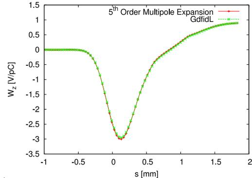
Figure 4: Longitudinal component of the wake-potential generated by a test charge in a simple test geometry, as calculated using GdfidL (green) and reconstructed via a multipole expansion to the 5<sup>th</sup> order (red). In this case, the files produced using GdfidL required 40 Mb of disk space, whereas the multipole coefficients used less than 10 Kb.
