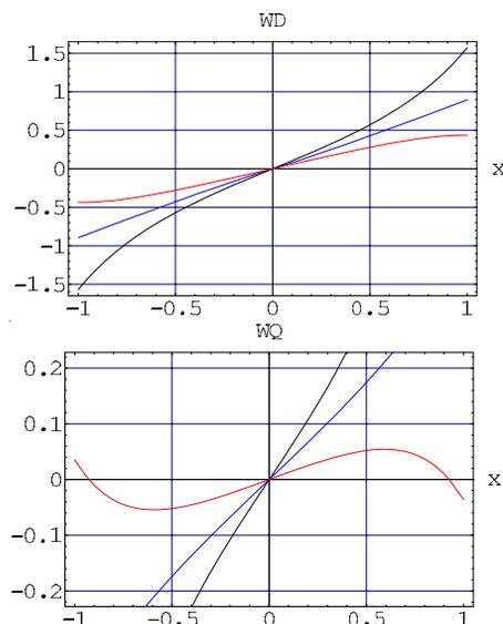
Figure 2: Dipole (left) and quadrupole (right) components of the wake field as a function of  $x_0/g$ ,  $x = 0$  and  $x_0 = 0$ ,  $x/g$  respectively, for  $(y - y_0)/g = 0$  (black), 0.5 (blue), 0.8 (red).
