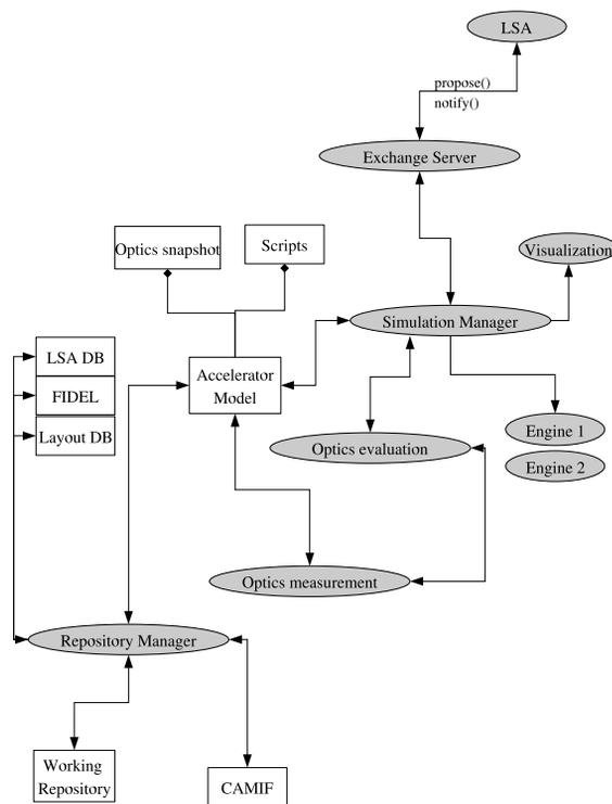
Figure 1: Software Architecture Design
