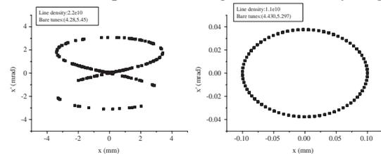
Figure 4: Trajectory in horizontal phase space at a peak proton line density of  $2.2 \times 10^{10} \text{ m}^{-1}$  [or  $N_b \approx 2 \times 10^{12}$ ] (left) and  $1.1 \times 10^{10} \text{ m}^{-1}$  (right) for the PS Booster with 4 electron lenses. At high intensity, the motion is destabilized by the newly excited structure resonance  $2Q_x = 8$ .
