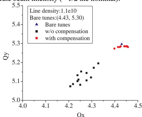
Figure 1: Tune footprint of the PS Booster computed for 12 test particles launched on a 2-D grid with initial start amplitudes ranging from  $1\sigma$  to  $2\sigma$ , without and with s.-c. compensation by 4 electron lenses.
