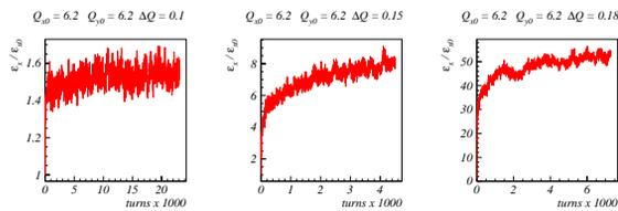
Figure 2: Emittance growth in a PS-like ring for a single constant electron lens adjusted to compensate a peak s.-c. tune shift  $\Delta Q^{SC}$  of 0.1 (left), 0.15 (center) and 0.18 (right). Head and tail particles are overcompensated, and they become transversely unstable for  $\Delta Q^{SC} > 0.13$ .
