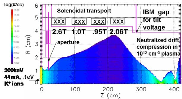
Figure 1: The STX simulation geometry is shown with the beam density near the time of peak simultaneous focus. From left to right are the ion source, diode, magnetic transport, IBM gap and plasma regions.
