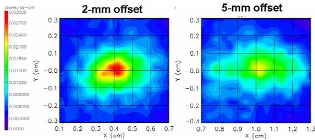
Figure 3: The energy deposition ( $J/cm^2$ ) from the compressed beam pulse is plotted for beam offset (a) 2 mm and (b) 5 m.
