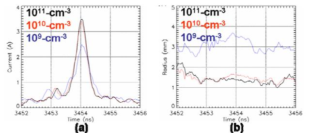
Figure 4: In a series of kinetic plasma simulations, the (a) compressed beam current and (b) edge radius at simultaneous compression are shown for the three plasma densities.
