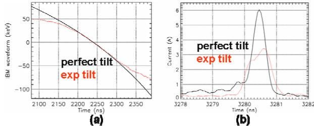
Figure 2: In (a), the experimental and perfect IBM voltage waveform are plotted. The resulting beam currents (27 mA initial) at  $z = 415$  cm are shown in (b).
