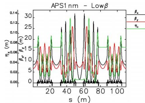
Figure 2: APS low-beta insertion 1-nm lattice Twiss parameters. Four insertions are placed symmetrically around the ring.
