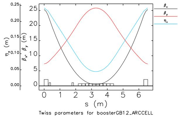
Figure 6: FODO cell for a booster low-emittance lattice upgrade.
