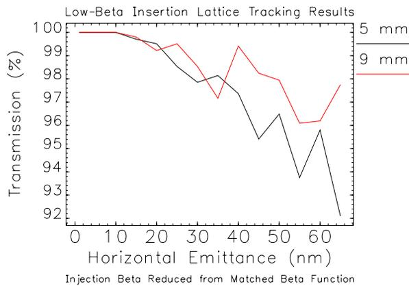
Figure 5: Tracking simulation results showing percent transmission for the low-beta insertion lattice with injection beta function reduced by a factor of five.
