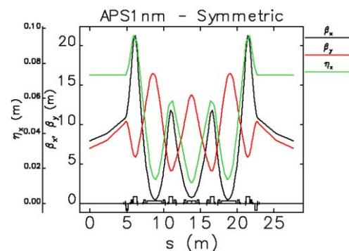
Figure 1: APS 1-nm symmetric lattice Twiss parameters.
