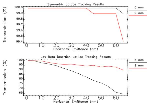
Figure 4: Tracking simulation results showing percent transmission in each lattice after 1000 turns. The different curves in the plots are for the two different bump heights. Both lattice error levels were adjusted so that the beta function beat was 5%.
