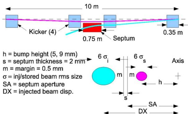
Figure 3: Injection straight section for APS 1-nm upgrade lattices. Shown is placement of kickers and septum as well as definitions of stored and injected beam displacement and septum thickness used in the tracking simulations.
