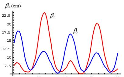
Figure 5:  $\beta$ -functions along the channel.
