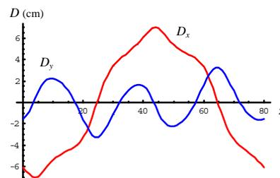
Figure 4: Dispersion functions along the channel.
