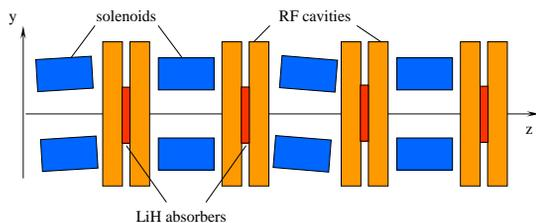
Figure 1: Schematic of the FOFO channel cell.
