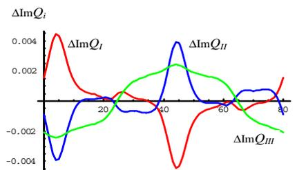
Figure 6: Change in cooling decrements vs wedge absorber position.
