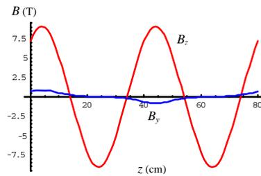
Figure 2: Magnetic field along the channel.
