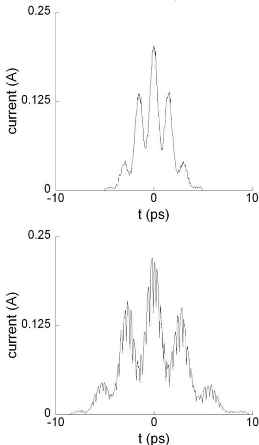
Figure 5: Density profiles of the 34 MeV beam just after the accelerator tank (top) and just after the wiggler (bottom). Note that density modulation remains in the beam at this energy.
