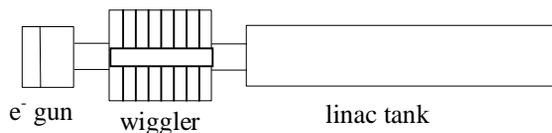
Figure 1: Accelerator system for low energy beams.
