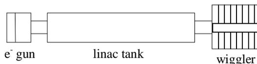
Figure 2: Accelerator system for higher energy beams.
