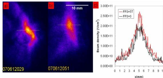
Figure 5: NDCX plasma neutralized beam profiles for axial compression (IBM: 25 kV, FCAPS 1 kV, FEP: 9 kV) with the final focus solenoid (a) powered, and (b) without powered; (c) profiles of the two images.
