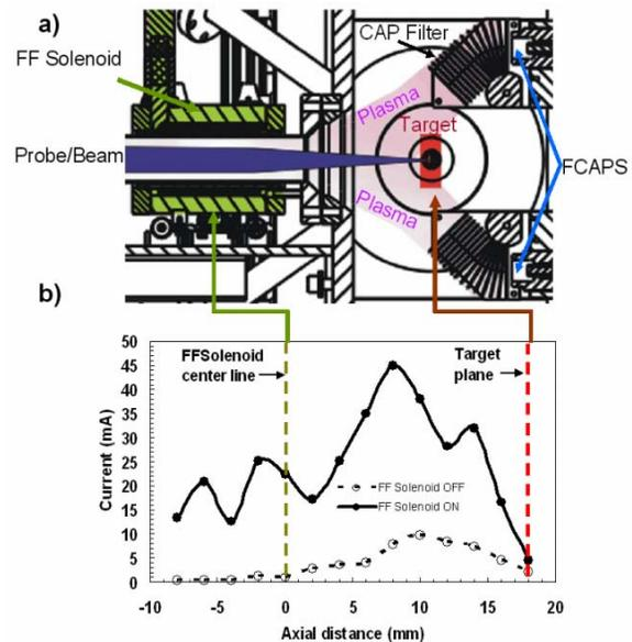
Figure 2. (a) A sketch of FCAP filters and the FFS in the target chamber, (b) measured plasma current (FCAPS: 1 kV discharge) with (for 4T) and without FFS powered.
