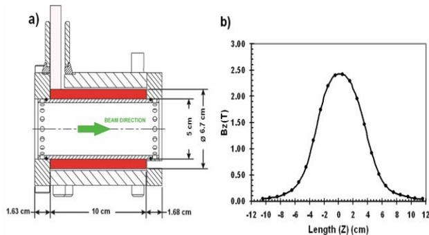
Figure 1. (a) A sketch of final focus solenoid and (b) characteristic magnetic field profile.
