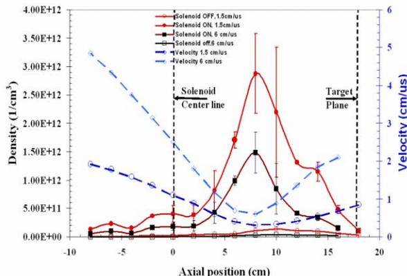
Figure 3: Inferred experimental axial plasma density distributions with and without magnetic field, for two initialized velocities in simulation. The dotted lines (blue in color) represent calculated velocities, initialized at 1.5 cm/ $\mu$ s and 6 cm/ $\mu$ s.
