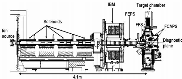
Figure 4: Sketch of the final focus solenoid (FFS) assembly integration with a  $K^+$  NDCX beamline.
