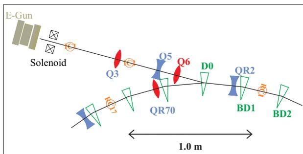
Figure 3: Collins-insertion geometry for matching/injection of low-current, space-charge dominated transport in UMER. See text for explanation of labels.
