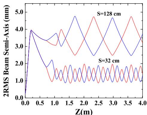
Figure 4: RMS Envelope matching calculations for low current (0.6 mA) in UMER with emittance-dominated ( $S=32$  cm), and space charge dominated ( $S=128$  cm) transport. See also Table I and Fig. 3.
