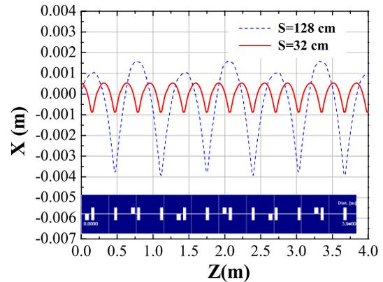
Figure 2: Closed orbits (shown over roughly 1/3 of the ring) obtained with the code WINAGILE for UMER lattices having full periods equal to  $S=128$  cm (broken curve), and  $S=32$  cm (solid curve). The vertical component of the earth's B-field is 0.4 G; the lattice for  $S=128$  cm is shown at the bottom.
