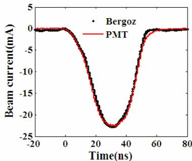
Figure 2: Current waveforms measured by Bergoz (dots) and PMT (the solid line).
