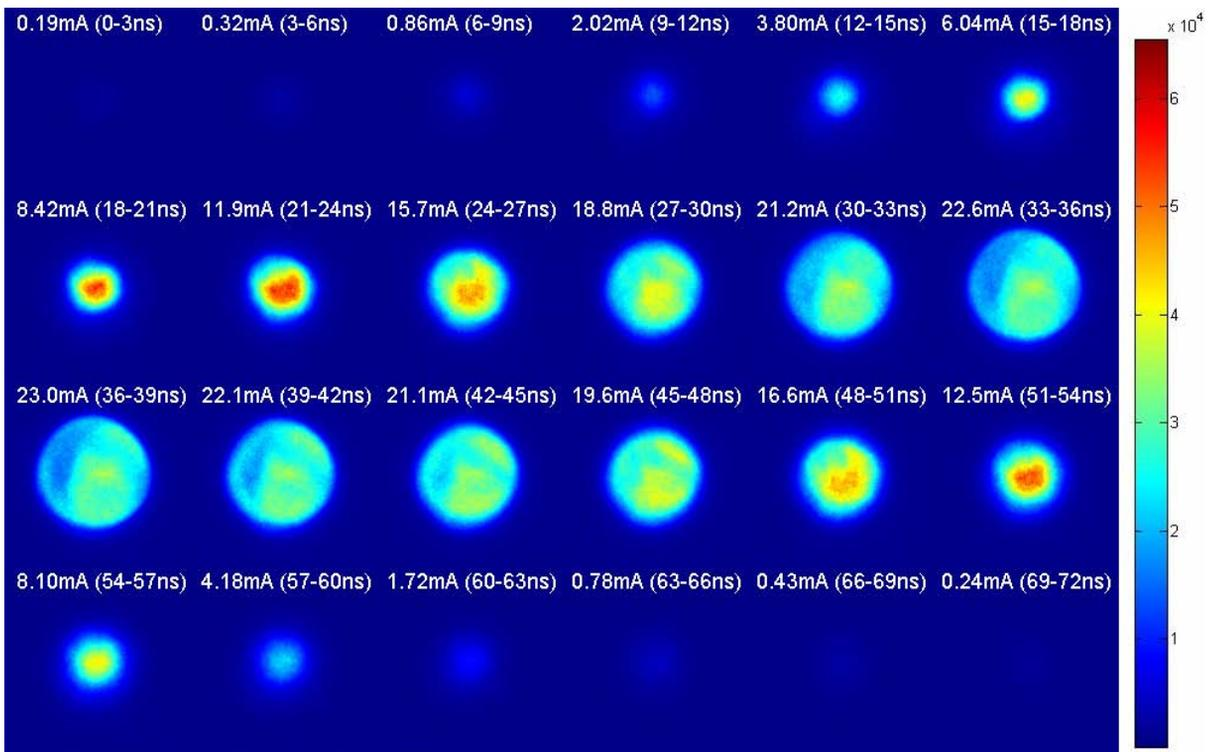
Figure 4: sliced beam images through the whole beam with a 3ns progressive gate on the ICCD camera
