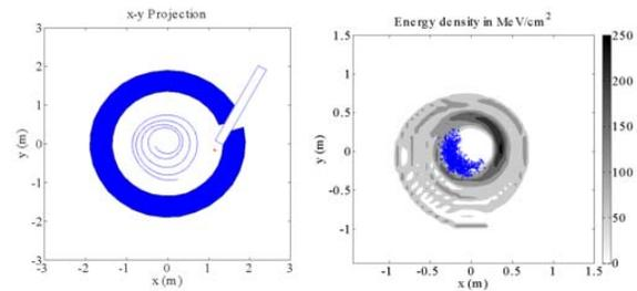
Figure 4: Trajectory of a single  $^{79}\text{Br}$  ion with an energy of 23 MeV/u after the degrader inside a sector-focused magnet filled with 180 mbar He (left). Energy deposition and stopped ion distribution (crosses) for a sector-focused magnet (right).
