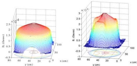
Figure 3: Magnetic fields obtained in a weakly focusing magnet (left) and a sector-field magnet (right), calculated with the TOSCA code.
