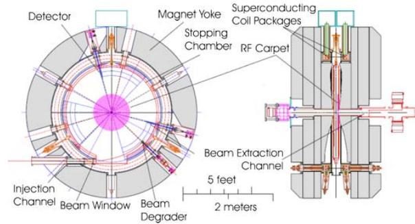
Figure 2: Design concept of the vertical superconducting magnet under consideration.
