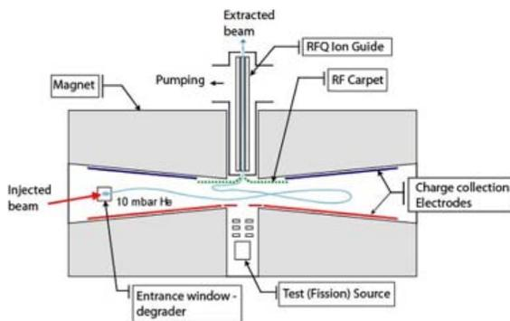
Figure 1: Schematic view of the cyclotron gas stopper showing the main components of the system. A cyclotron-type focusing magnet contains a vacuum chamber filled with helium at low pressure, a beam degrader, charge collection electrodes, and an RF carpet for ion extraction.
