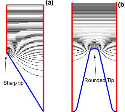
Figure 3: Magnetic field lines penetrating in a groove. A half period of a groove with sharp tip is shown in (a) and
