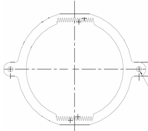
Figure 7: Sketch of the beam pipe with grooved surface in a dipole magnet.
