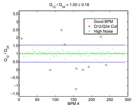
Figure 2: Invariant ratio,  $Q_{12}/Q_{34}$ , calculated from the Four independent orbits extracted from PEP-II HER BPM buffer data taken on April 27, 2007. The blue horizontal lines show the 3 standard deviations.
