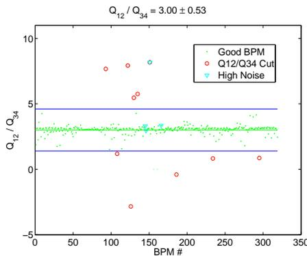
Figure 1: Invariant ratio,  $Q_{12}/Q_{34}$ , calculated from the Four independent orbits extracted from PEP-II LER BPM buffer data taken on April 22, 2007. The blue horizontal lines show the 3 standard deviations.
