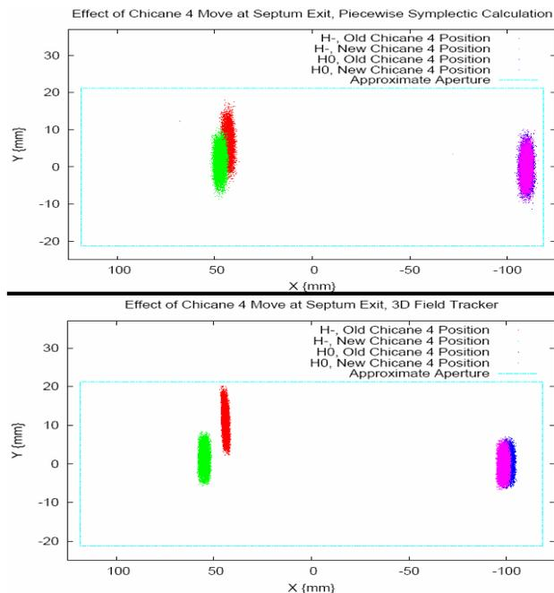
**Figure 2.** Piecewise symplectic (top) and 3D (bottom) beams at the exit of the injection dump septum.  $H^0$  and  $H^-$  components are on the right and left, respectively. Red and blue correspond to original dipole four position, and green and pink to the moved dipole four. The blue rectangle shows the approximate aperture position.
