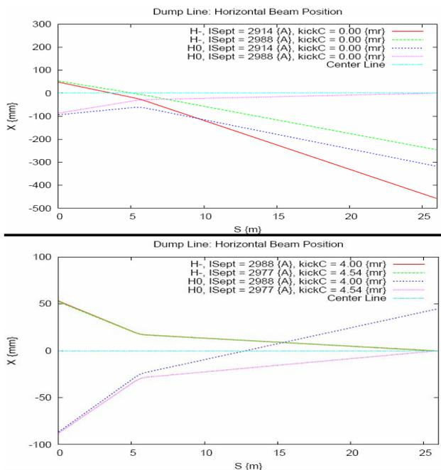
Figure 3.  $H^-$  and  $H^0$  horizontal beam centroids during the tuning process.
