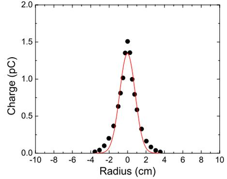
Figure 3: Radial profiles of the trapped barium ions in the PTSX device. The red curve is a Gaussian fit to the measured signals.
