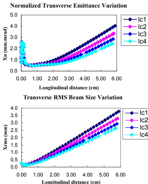
Figure 2: Beam properties in and after dc guns for Gun lc1 to lc4: (a)  $X_n$  variations; (b)  $X_{rms}$  variations.
