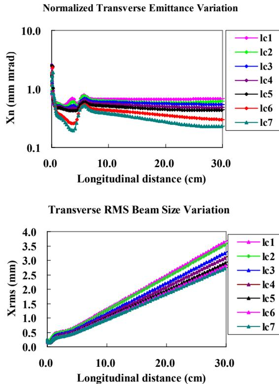
Figure 3: Beam properties for the entire dc/rf guns. The dc guns are labeled with Gun lc1 to lc7: (a)  $X_n$  variations; (b)  $X_{rms}$  variations.
