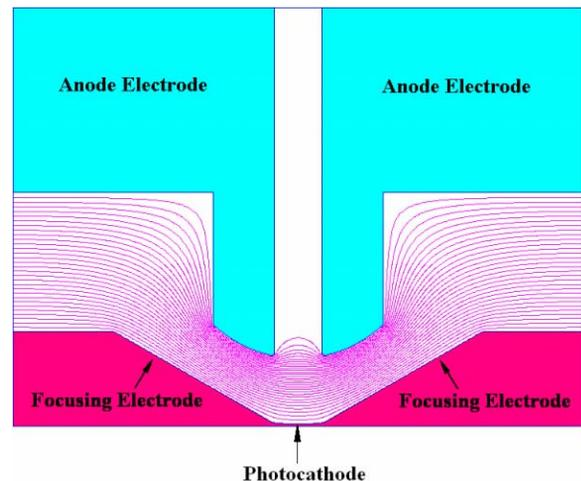
Figure 1: Diagram of the dc gap with SUPERFISH field plotted.
