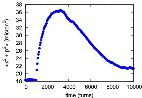
Figure 3: Evolution of the total transverse action for a marginally stable beam.
