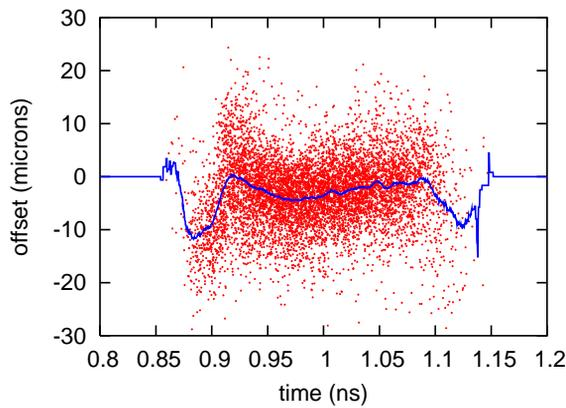
Figure 2: Transverse offset versus position along the bunch for a marginally unstable beam .
