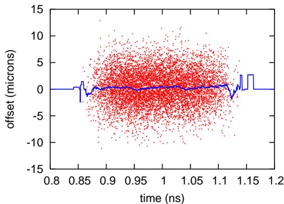
Figure 4: Transverse offset versus position along the bunch for a marginally stable beam .
