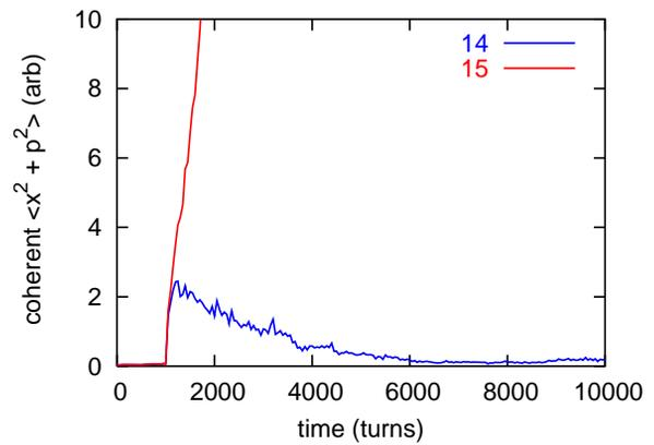
Figure 5: Comparison of coherent amplitude for stable and unstable beams.
