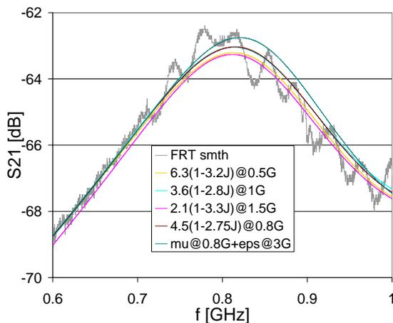
Figure 6: Matching of the S21 with different mu-values
