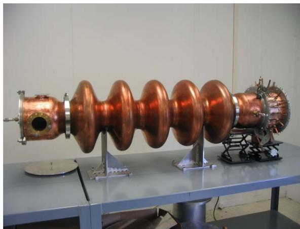
Figure 1: Cu cavity with HOM absorber
