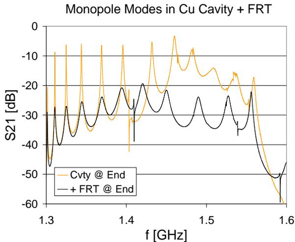
Figure 3. Monopole modes w/wo ferrite absorber
