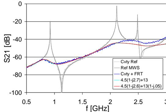
Figure 8: Simulation of pillbox cavity w/wo ferrite
