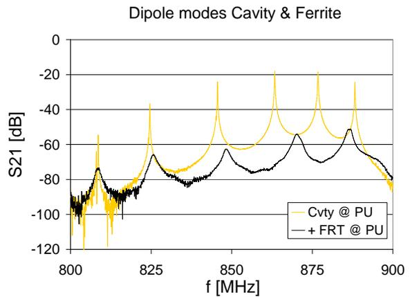
Figure 4: Dipole modes w/wo ferrite absorber
