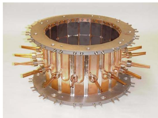
Figure 5: Absorber model with ferrite tiles
