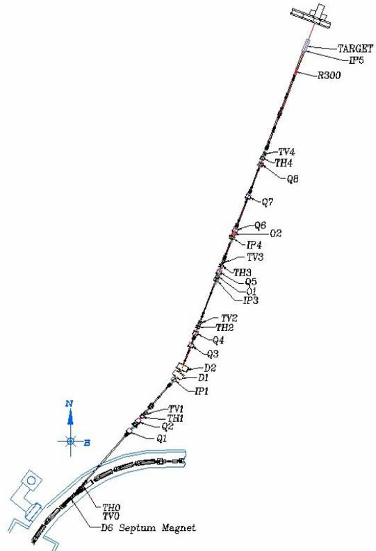
Figure 2: Drawing of the NSRL line. Shown are the main magnets and corrector magnets and the instrumentation packages (IP).
