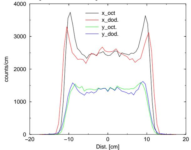
Figure 6: Calculated horizontal and vertical projections of the beam distribution at the target; with octupoles (black/green) and dodecapoles (red/blue). The counts for the vertical distributions have been scaled down by a factor of 2, for the curves to be separated for clarity purposes.
