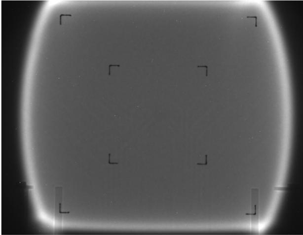
Figure 4: A uniform beam distribution at the target. The inner and outer tic marks correspond to distances of 10 cm and 20 cm respectively.
