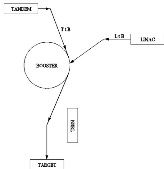
Figure 1: Schematic diagram of the NSRL line in relation to the Booster synchrotron, which accelerates the ions, the LINAC, which provides a proton beam, and the Tandem accelerator, which provides beams of many ion species.
