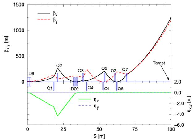
Figure 3: The horizontal- and vertical-beta ( $\beta_{x,y}$ ) and dispersion ( $\eta_{x,y}$ ) functions along the NSRL beam transport line. The rectangular blue boxes in the figure correspond to the magnetic elements of the line. The label D20 in the figure designates the two dipoles D1 and D2 of Fig.1.
