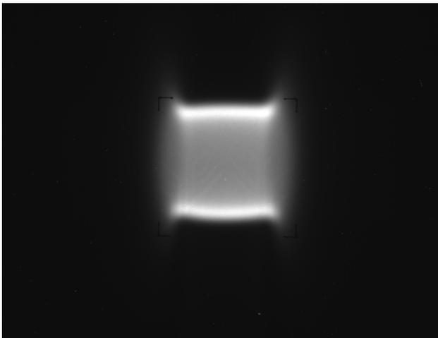
Figure 5: A uniform beam distribution at the target. The size of the area where the beam is uniform is  $\sim 8 \times 8 \text{ cm}^2$ .
