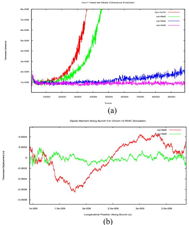
Figure 3: (a) The transverse coherence evolution for head-tail mode. The vertical axis is the coherence as defined in [2]. The red green blue and purple curve are for bunch population of  $10^{10}$ ,  $8 \times 10^9$ ,  $5 \times 10^9$  and  $4 \times 10^9$  respectively. (b) A snapshot of the transverse displacement along the bunch. The red and green curves are for  $8 \times 10^9$  and  $5 \times 10^9$  ions per bunch.
