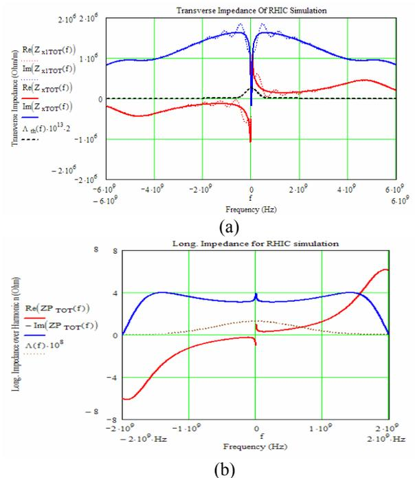
Figure1: (a) RHIC Transverse Impedance. The dot curves are for step form bpm impedances. (b) RHIC Longitudinal Impedance over harmonic  $Z_{||}/n$ . The Gaussian curves in both graphs roughly show the range of beam spectrum.
