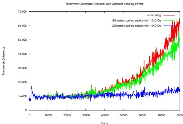
Figure 5: The Transverse Coherence Evolution With varies E-cooling Parameters. The bunch population is  $6 \times 10^9$  and the chromaticity is 2.
