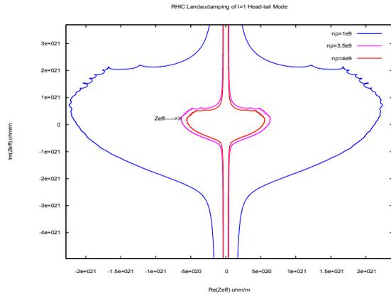
Figure 4: Stability threshold contours for  $\mu = 1$  head-tail mode. The blue, purple and red curve are the stability threshold contours for bunch population of  $10^9$ ,  $3.5 \times 10^9$  and  $4 \times 10^9$  respectively. The 'X' marks the effective impedance calculated directly from the definition, Equation (3), using the impedance shown in Figure 1.
