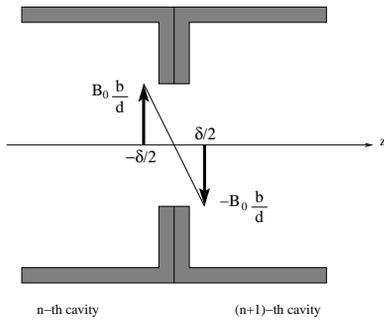
Figure 2: Field gradient between two contiguous cavities
