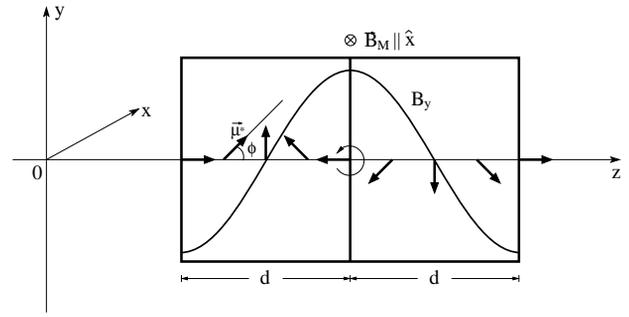
Figure 3: Display of how two  $\pi$ -out-of-phase cavities can yield a non null energy exchange if combined with a  $180^\circ$  spin precession here sketched.
