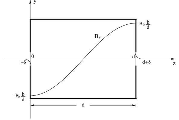
Figure 1: Edge fields at both ends of a single cavity
