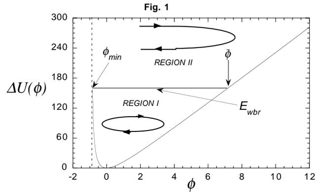
Figure 1: Oscillating (*I*) and wave breaking (*II*) regions for the electric potential at  $\psi = 0$ .
