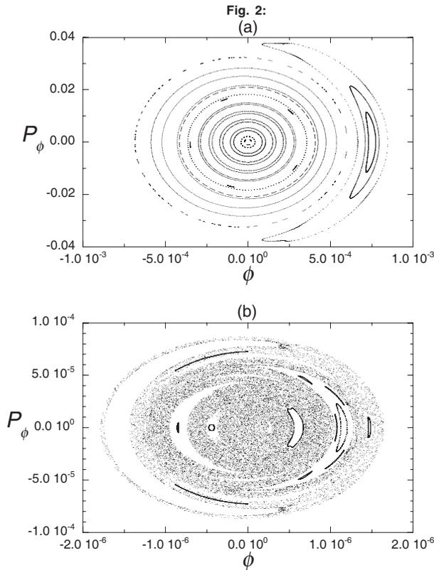
Figure 2: (a) Phase plot near the modulational instability threshold, with  $\eta = 1.00001\eta_*$ ; (b) phase plot after the inverse tangency, with  $\eta = 1.0001\eta_*$ .  $\epsilon = 10^{-11}$ .
