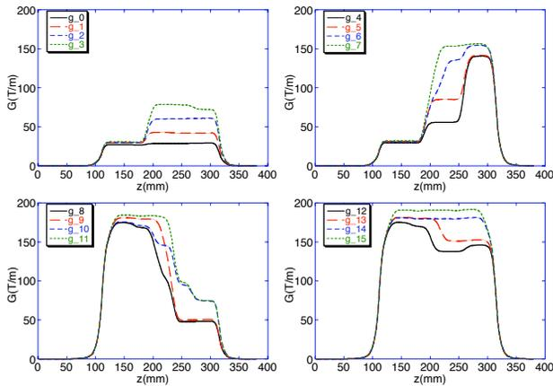
Figure 5: Longitudinal field distributions at 15 steps.
