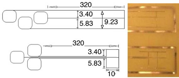
Figure 4: Tangential coils that enable three values of opening angle:  $\pi/13$ ,  $\pi/7$  and  $(1/12+1/7)\pi$ . Short coil (bottom) will be used to measure the longitudinal field distribution. The dimensions are in mm.
