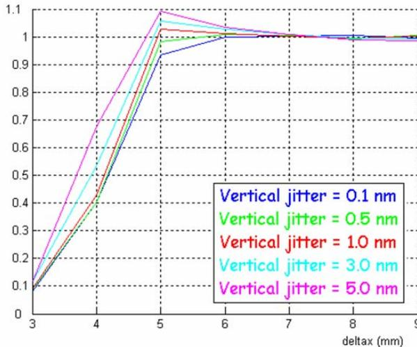
Figure 4: Relative luminosity ( $L_0/L_{\text{with KINK}}$ ), for a “Guinea-Pig + DIMAD 50000 macro-particles” modelling versus distance between bunches at the FPC (Nominal parameter at 500 GeV center of mass).
