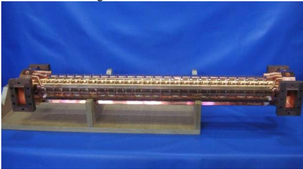
Figure 6: 10 MeV structure after brazing.
