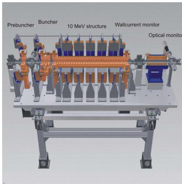
Figure 2: 3D model of the 10 MeV structure including the bunching system.
