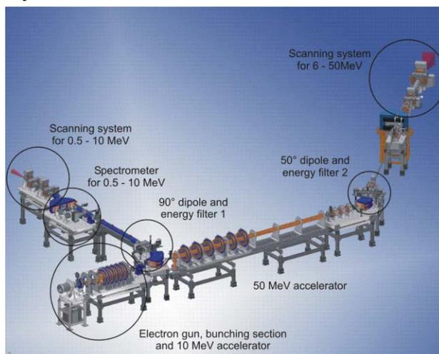
Figure 1: 3D model of the PTB accelerator layout.
