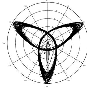
Figure 7: Beadpull measurement at the 50 MeV structure after tuning.
