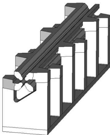
Figure 1: A 4-rod  $\lambda/2$  RFQ simulation model with six stems and plain electrodes.
