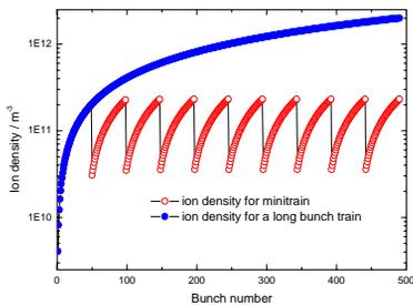
Figure 3: Ion density versus bunch number for 10 bunch trains in fill pattern case A.
