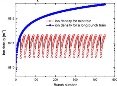
Figure 5: Ion density versus bunch number for 10 bunch trains in fill pattern case C.
