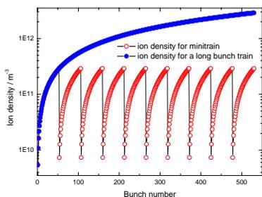
Figure 4: Ion density versus bunch number for 10 bunch trains in fill pattern case B.
