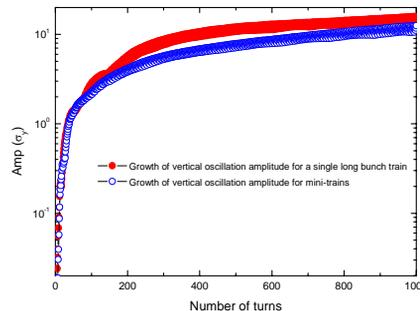
Figure 6: Growth of vertical oscillation amplitude for a single bunch train and mini-trains, respectively with fill pattern A for a CO partial pressure of 1 nTorr.
