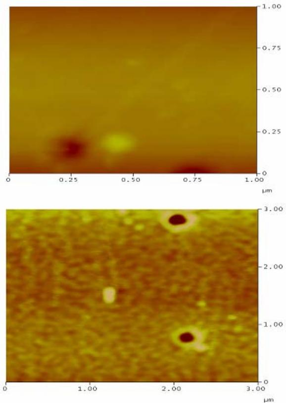
Figure 3: Two dimensional view of AFM micrograph of PMMA surface with 10 keV electron beam (a) Pristine and (b) irradiated at fluence  $1 \times 10^{16} e/cm^2$
