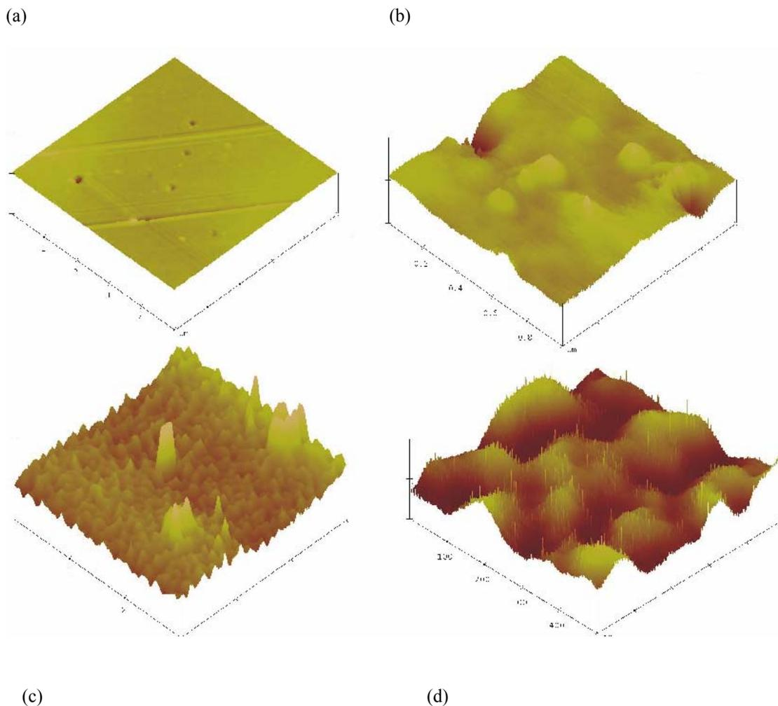
Figure 4: AFM images of (a) Pristine PMMA, (b) irradiated with fluence  $4 \times 10^{14} \text{ e/cm}^2$ , (c) at fluence  $4 \times 10^{15} \text{ e/cm}^2$  and (d) at fluence  $1 \times 10^{16} \text{ e/cm}^2$
