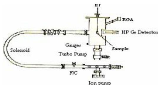
Figure 2: The sketch diagram of linear electron beam accelerator
