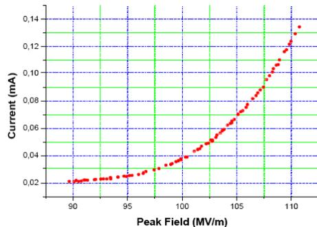
Figure 3: Dark current as a function of gun peak field.
