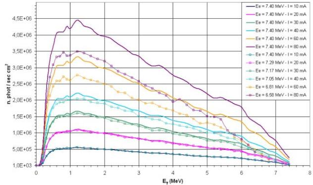
Figure 3: Comparison between energy spectra obtained for fixed and not fixed magnetron power cases.
