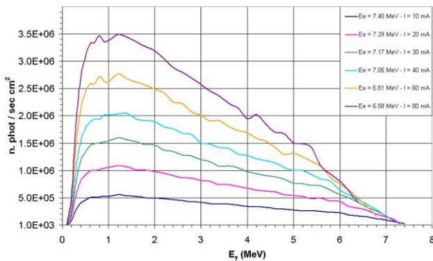
Figure 2: Energy spectra, as photons/cm<sup>2</sup> s vs MeV, of the bremsstrahlung beams obtained selecting different electron energies.
