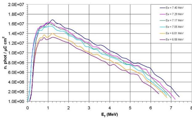
Figure 1: Energy spectra, as photons/cm<sup>2</sup>μC vs MeV, of the bremsstrahlung beams obtained selecting different electron energies.
