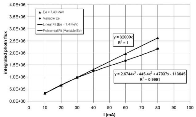
Figure 4: Comparison between integrated x-ray flux as a function of the electron current for fixed and not-fixed magnetron power cases.
