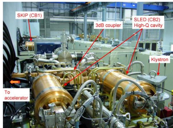
Figure 4: RF pulse compressor (SLED) at CB2.
