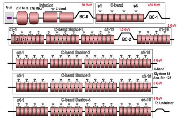
Figure 1: Computer Image of XFEL facility in SPring-8 site, and rf acceleration design of XFEL .
