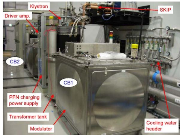
Figure 5: Modulators and klystrons.
