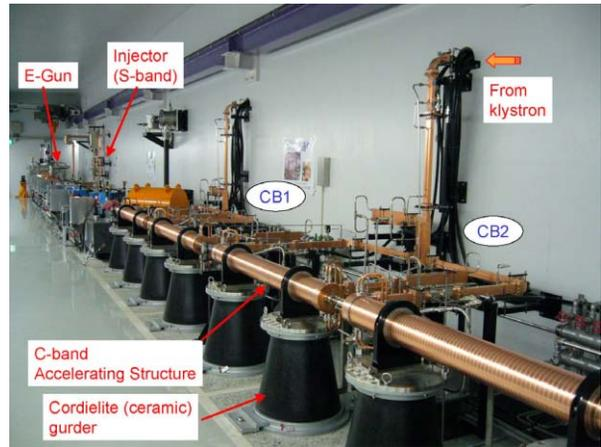
Figure 3: C-band accelerating structure in the tunnel.
