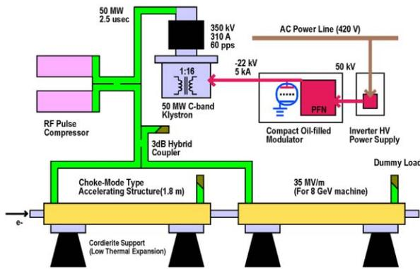
Figure 2: C-band accelerator system.
