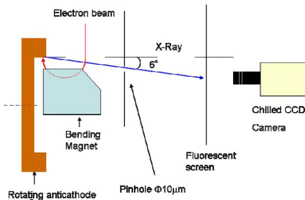
Figure 5: A schematic view of X-ray measurement system.
