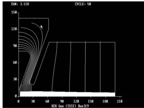
Figure 2: Output of EGUN simulation for the case of the extraction voltage of 60 kV, grid voltage of 3 kV and the cathode diameter of 2 mm.
