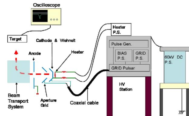
Figure 3: System configuration of test stand.
