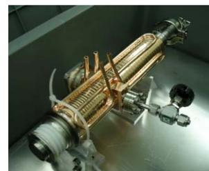
Figure 6: The accelerating tube with gun and RF window
