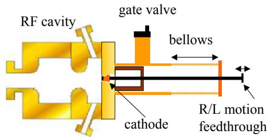
Figure 2: Schematic view of RF cavity with a cartridge-type photocathode system.
