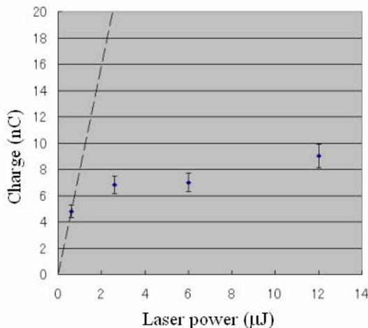
Figure 4: Charge vs laser power. The line is estimated the same QE of 3.5%.
