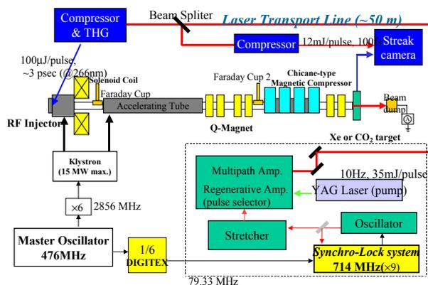
Figure 1: Experimental setup of sub-picosecond pump and probe system.
