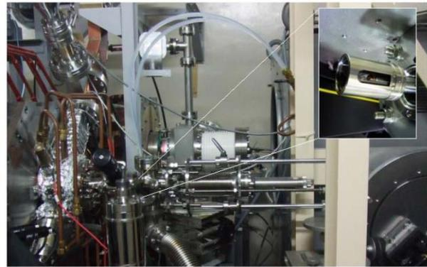
Figure.3 Picture of the system. The cathode is installed into the cartridge case and set at the head of feedthrough.
