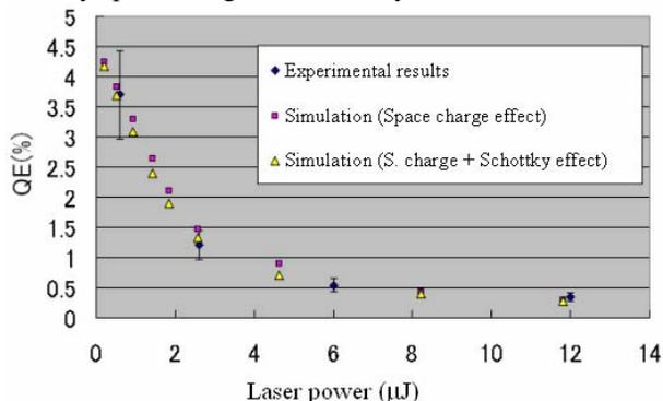
Figure 5: Charge vs laser power. The line is estimated the same QE of 3.5%.
