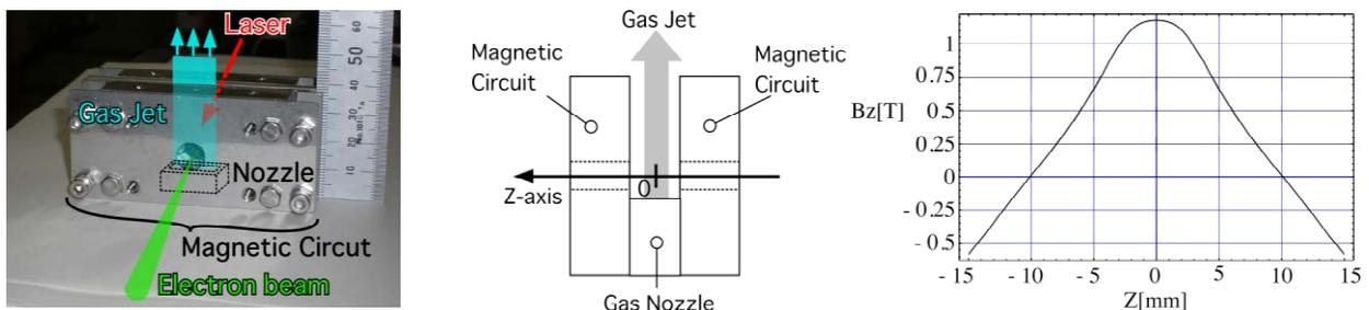
Figure 5: Calculated magnetic flux density of the magnetic circuits on the laser axis and picture of magnetic circuits which generate 1.0 T magnetic field.
