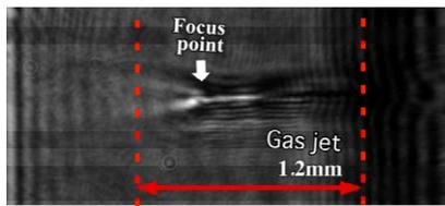
Figure 6: Typical shadowgraph image of the plasma at 1.2ps before the main pulse for  $N_{\text{He}}=4.2 \times 10^{19} \text{ cm}^{-3}$ ,  $B=1.0\text{T}$  and a laser power of 12 TW.
