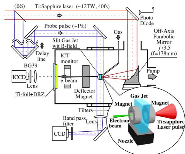
Figure 2: Experimental setup. A supersonic slit nozzle with ring magnets is magnified in the inset.
