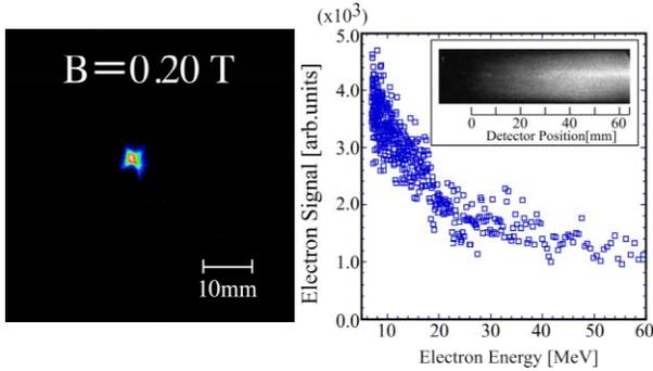
Figure 3: (a) Typical image of electron deposition on the DRZ screen, and (b) typical energy spectra of accelerated electrons. The image on the screen is shown in the inset.  $N_{He}=4 \times 10^{19} \text{cm}^{-3}$ ,  $B=0.2 \text{T}$  and the laser power is 12 TW.
