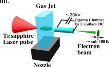
Figure 1: The schematic illustration of the plasma cathode experiments with two steps acceleration mechanism.
