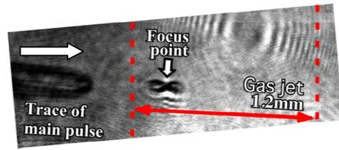
Figure 4: Typical shadowgraph image of the plasma at 1.2ps before the main pulse for  $N_{He}=4.2 \times 10^{19} \text{cm}^{-3}$ ,  $B=0.2 \text{T}$  and a laser power of 12 TW.
