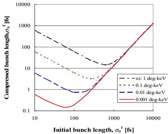
Fig. 2. Dependence of final compressed bunch length,  $\sigma_z^f$ , on initial bunch length at linac exit,  $\sigma_z^i$ , and longitudinal emittance,  $\epsilon_z$ .
