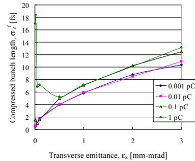
Fig. 4. Dependence of compressed bunch length,  $\sigma_z^f$ , on transverse emittance,  $\epsilon_x$ , and bunch charge.
