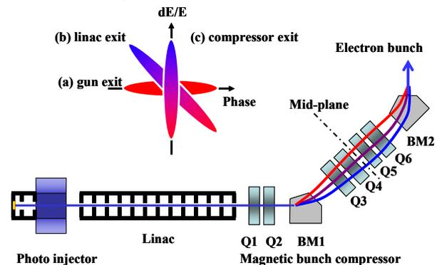
Fig. 1. Photocathode femtosecond electron linac and phase space distributions of bunch at the exit of the gun (a), at the exit of the linac (b), and at the exit of the compressor (c).
