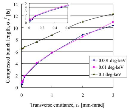
Fig. 3. Dependence of compressed bunch length,  $\sigma_z^f$ , on transverse emittance,  $\epsilon_x$ , and longitudinal emittance,  $\epsilon_z$ .
